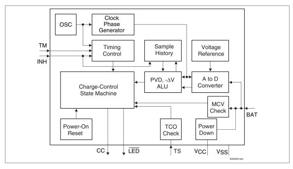
Figure 3. Block Diagram
