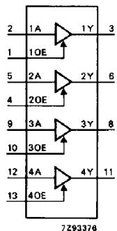
Fig. 4 Functional diagram.
