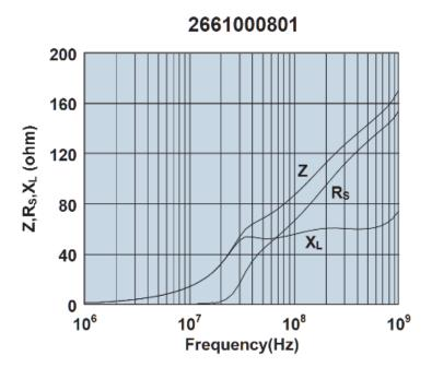
Impedance, reactance, and resistance vs. frequency.
